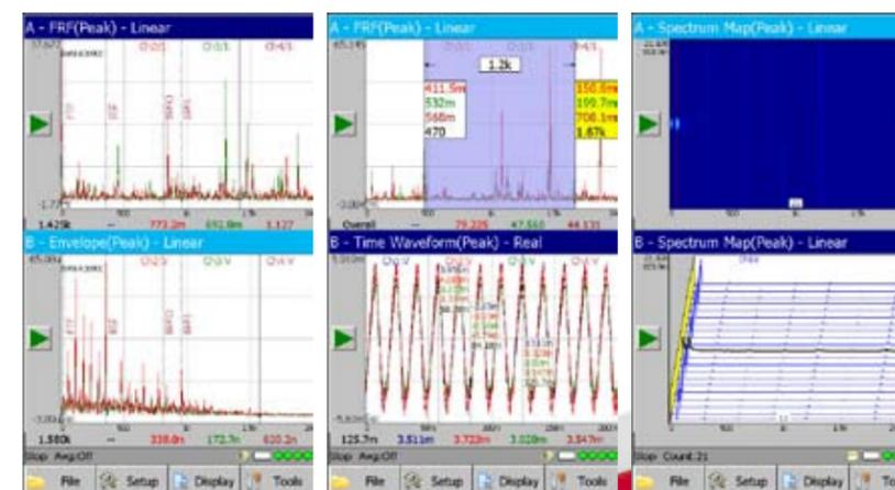
Fieldpaq II's FFT program also supports bearing vibration analysis as a standard feature. By taking advantage of demodulation technology, one may see the fault frequencies of a bearing on a demodulated spectrum at its early stage of damage. Fieldpaq II's demodulated spectrum uses a wavelet based Hilbert Transform algorithm, which shows clear spectral pattern(s) and low levels of sidebands.
