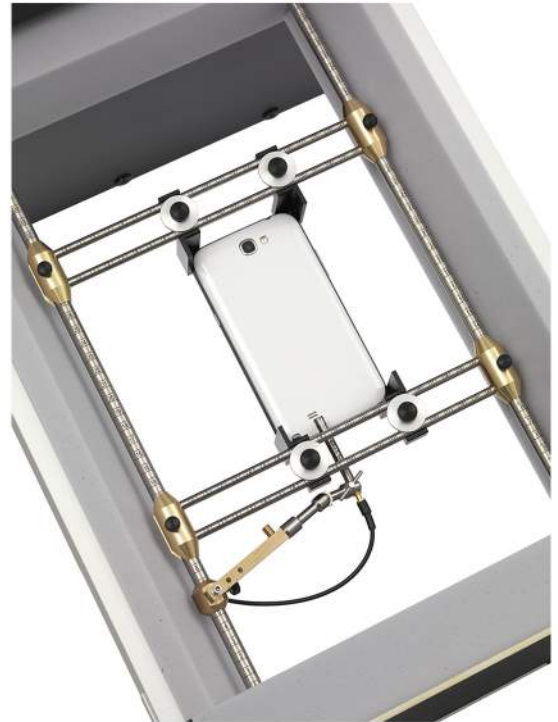
Test jig with DUT and measurement microphone.
